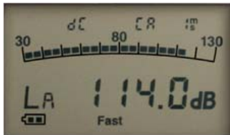
Calibration mode using built-in 1 kHz sound source
